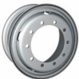
Wheels with 5° bead seats for trucks, buses, low-bed semi-trailers, trailers and special purpose vehicles
